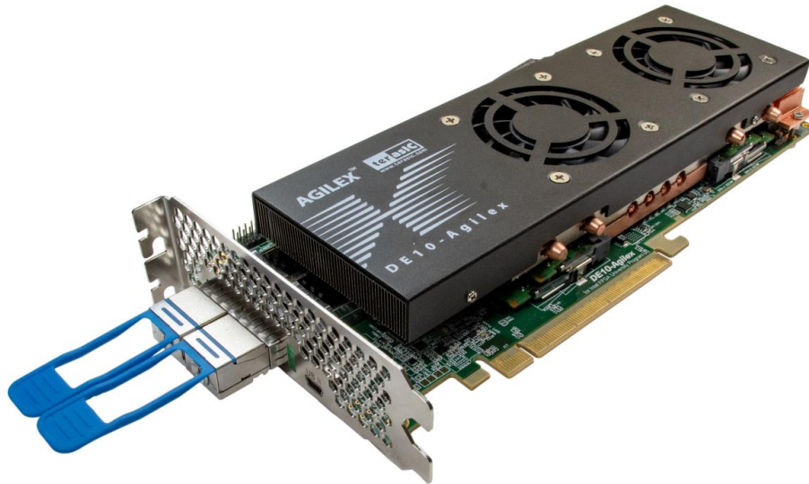
Figure 9-2 QSFP-DD Transceiver Loopback Test in Progress
