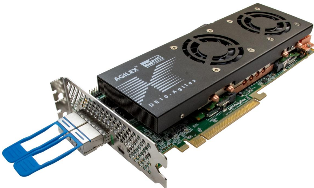
Figure 9-9 Setup QSFP28 or QSFPDD loopback fixture
