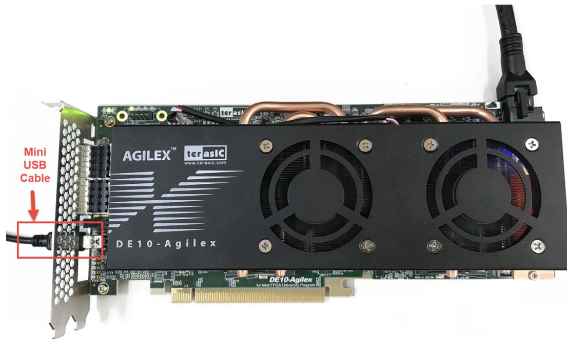
Figure 10-2 Connection setup for using dashboard system
